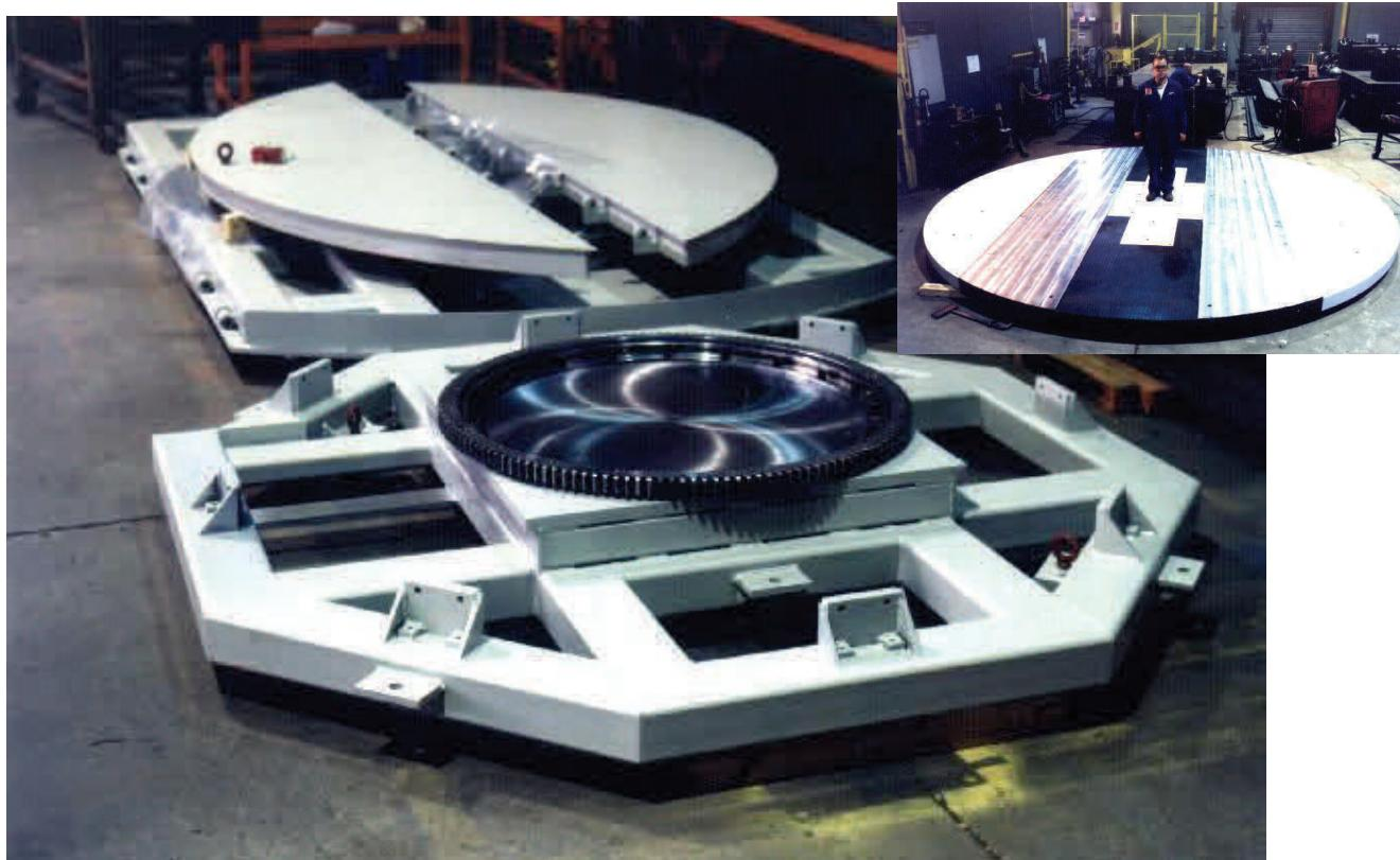
**H**andling Specialty custom engineered and manufactured a rotator that was used in an automotive laboratory wind testing system, where different car models were driven onto the rotator and then turned to face the wind tunnel.
