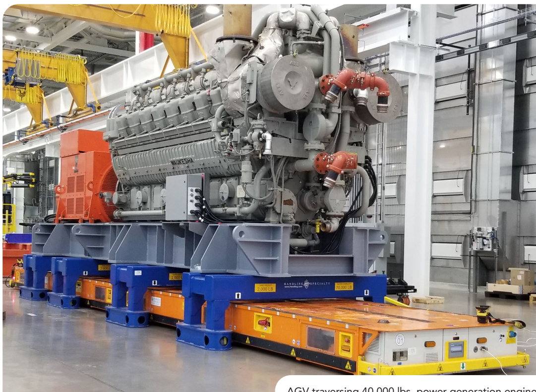
AGV traversing 40,000 lbs. power-generation engine.
