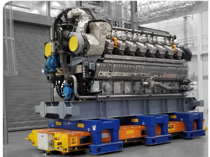
AGV traversing 40,000 lbs. power-generation engine.
